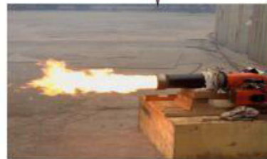
Oil to Heat the Reactor
