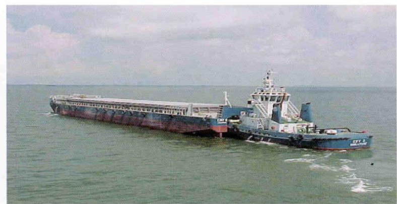
Composite unit of Tug & Barge
