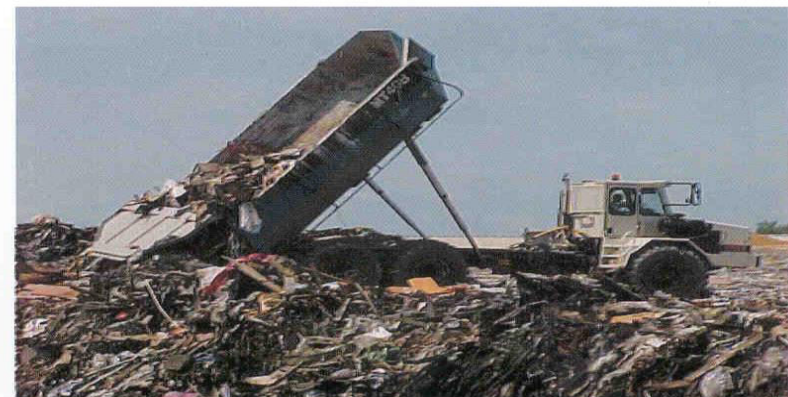
Tipping Waste at Landfill Cell
