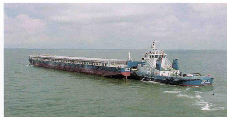
Composite unit of Tug & Barge
