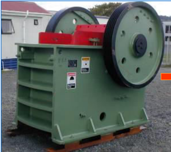
Phase 1: Pre-crush to 40mm
